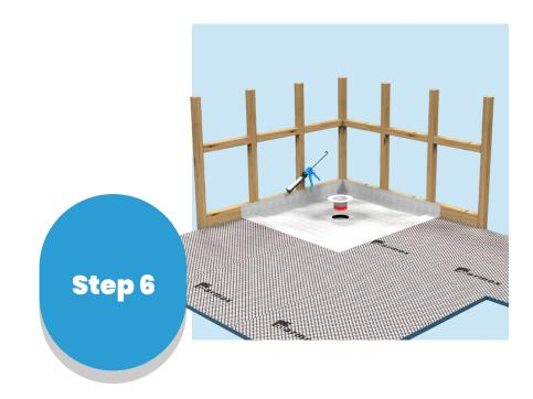
6. Apply a bead of polyurethane on the stainless-steel plate and plumber's glue to the drainpipe. Then fix the drainage flange in position and apply a bead of polyurethane to the outside of the flange.
