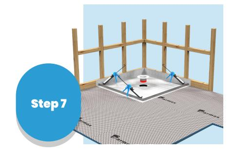
7. Fix a suitable height aluminum angle to the outside line of the MARMOX underlay or shower stone as a water stop using polyurethane adhesive.
