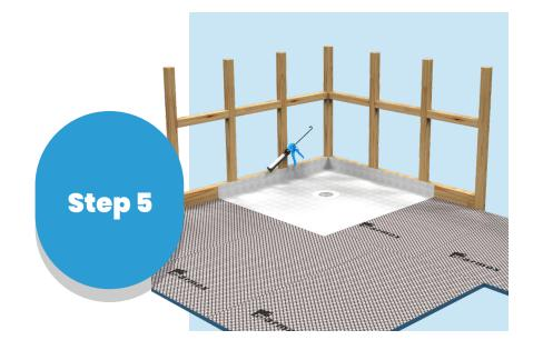
5. Use the same adhesive to glue the loose ends of the fleece to the wall and the floor.
