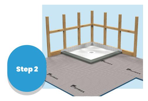
2. Place the underlay in position, apply downward pressure on the underlay and check for level. Use the same adhesive to glue the loose ends of the fleece to the wall and the floor.
